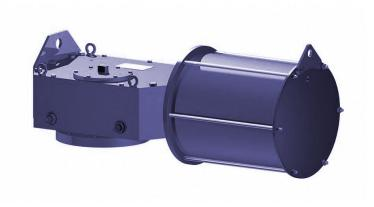
The Scotch Yoke mechanism allows the HD actuators to be suitable for high torque valve applications, due to the actuators highest output torque at the cylinder start and spring ending position, closely following a ball valves torque profile.
